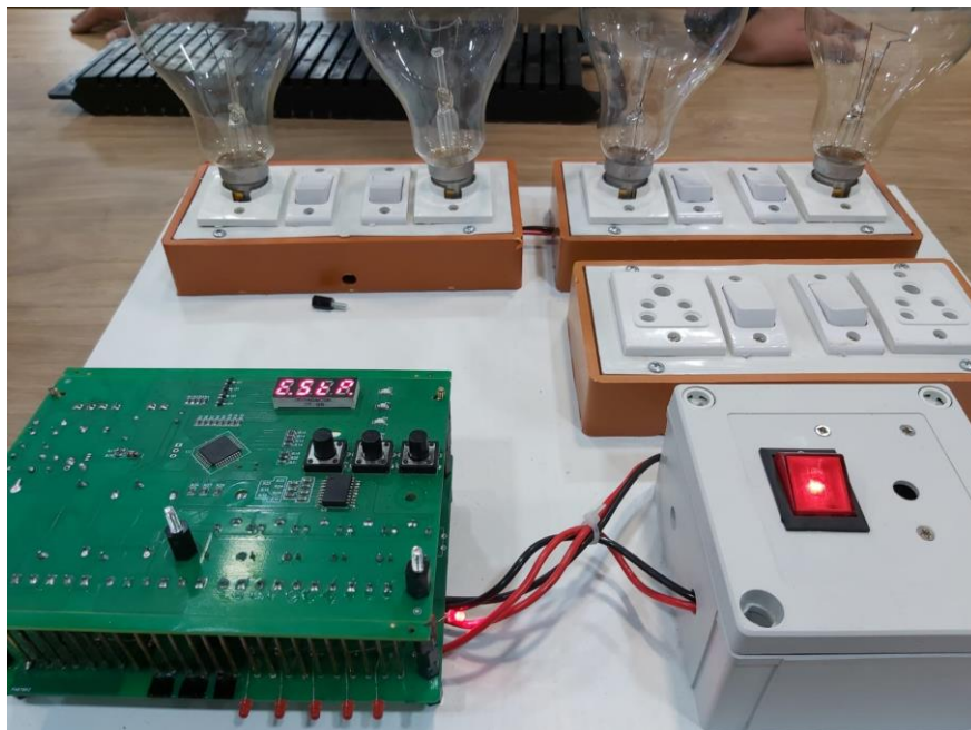
Figure 33 Test Setup for PCB
